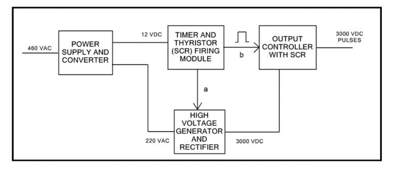
Power supply and converter consists of power step down transformers for and rectifiers. It receives 460-480 volts AC at 50/60Hz and produces outputs of 220 volts AC 50/60Hz (supplied to high voltage generator and rectifier) and 12 volts (supplied to timer and thyristor firing module).
