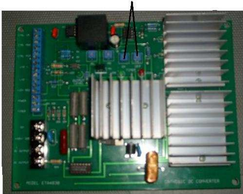
Figure 5: DC-DC Down Converter
