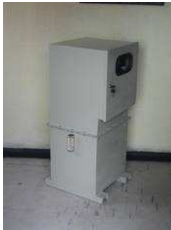
Angular view of rectifier showing the oil level gauge.
